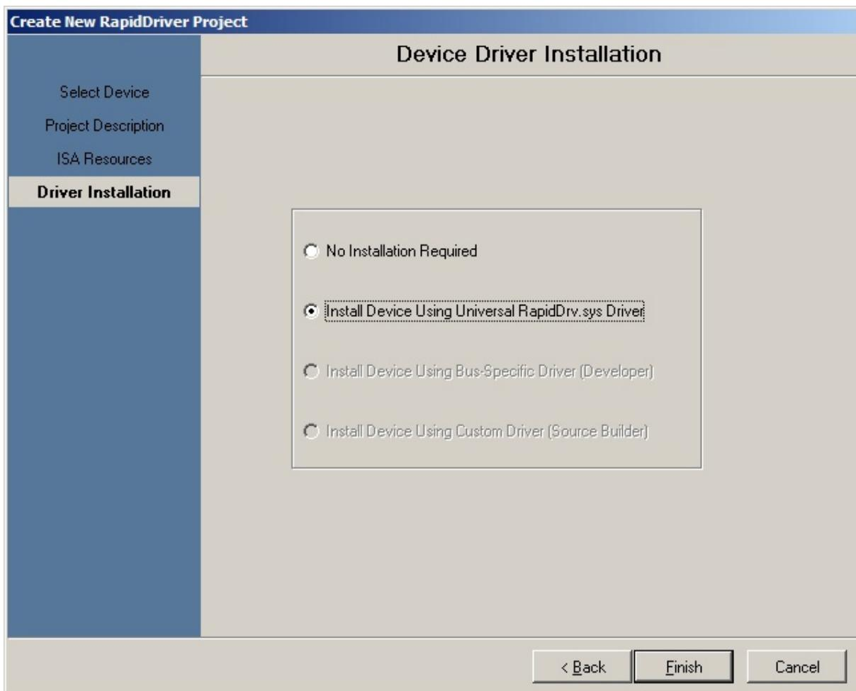
Select a driver which should be installed after you press the "Finish" button. You may also select the "No installation required" alternative and install the driver later by pressing of the
